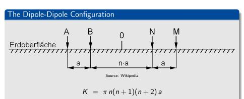
Particularly suitable for profiling of small-scale structures, but a requires high power input.
