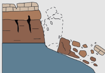
Rotational slide (Slump)
