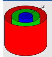
Flow in radial direction requires that p(x, y, z, t) only depends on  $r = \sqrt{x^2 + y^2}$  and t; use p(r, t) instead of p(x, y, z, t).
