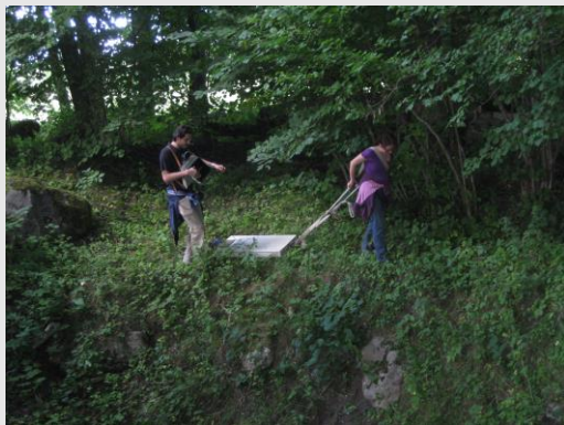
Fieldwork with ZOND 100 and 300 MHz antennas
