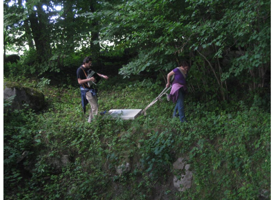
Fieldwork with ZOND 100 and 300 MHz antennas
