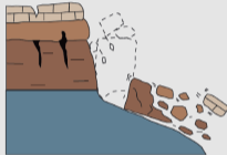
Rotational slide (Slump)
