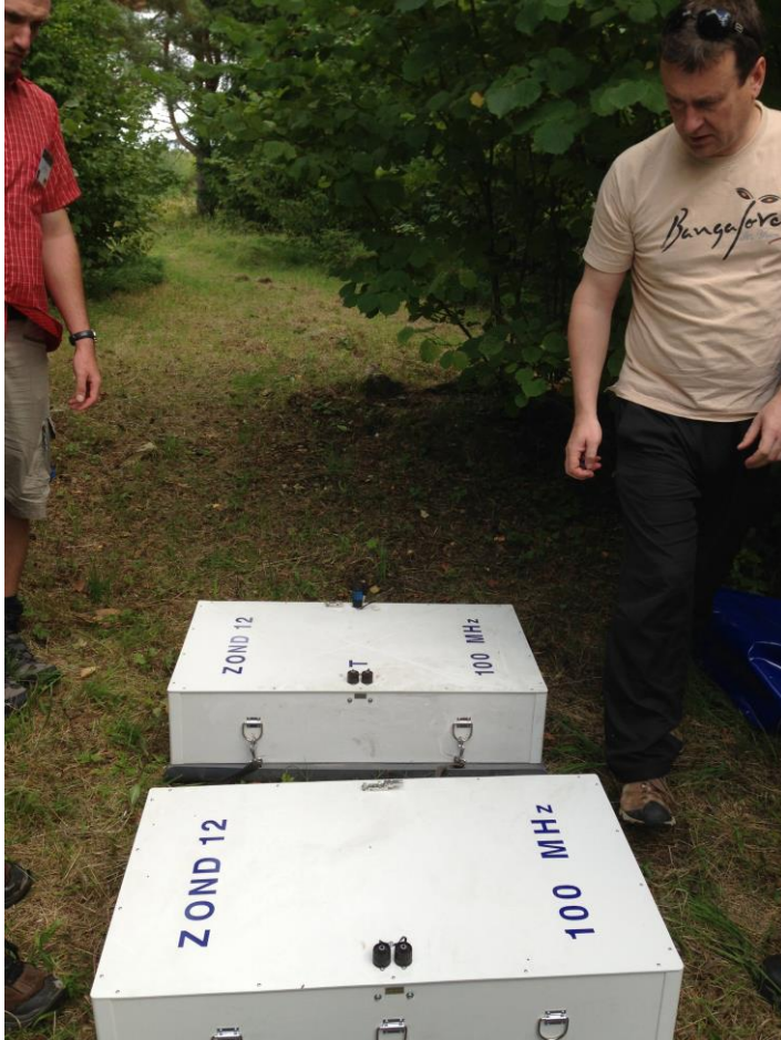
Fieldwork with ZOND 100 and 300 MHz antennas
